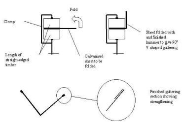
**Figure 3a:** folding galvanised steel sheet to make V-shaped guttering
