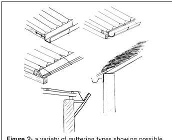
**Figure 2:** a variety of guttering types showing possible fixings
