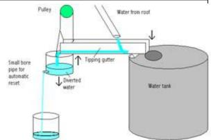
Figure 7a: Tipping gutter mechanism
